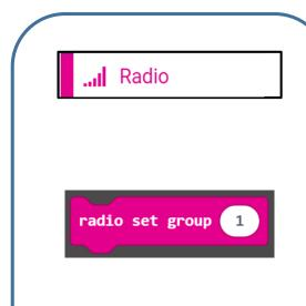
Allows communication between micro:bits via radio that have the same group ID
